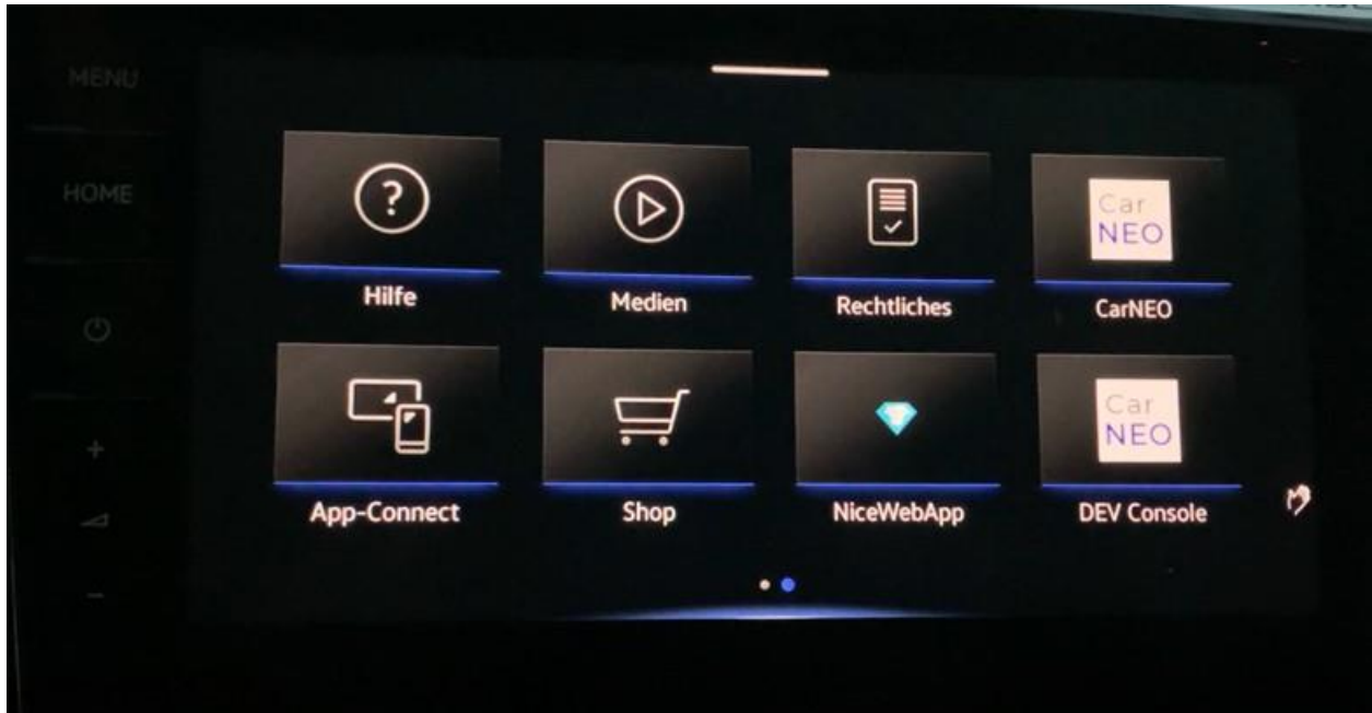
Figure 10: CarNEO as in-car App (photo of the infotainment system in the test vehicle, CarNEO is the prototype in-car app for managing the consents and CarNEO dev Console is for debugging and logs viewing)
